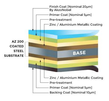
The substrate is made from AZ 200 alloy coated steel sheets. AZ is an alloy comprising 55% Aluminium, 43.5% Zinc and 1.5% Silicon. AZ 200 refers to the coating mass in g/m<sup>2</sup> on both sides.
