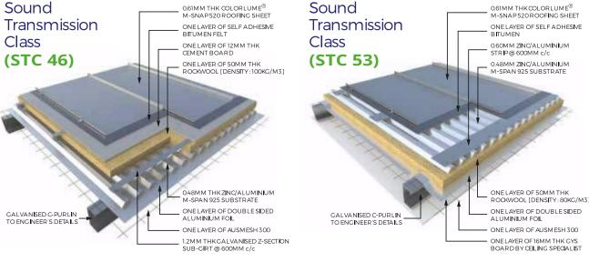
\* Ausmesh 300 safety roof mesh is designed to support insulation and to help prevent construction roof workers from falling.
